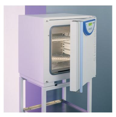
The device STERICELL® serves for hot-air sterilization of medical devices and materials with pre-set temperature and time parameters.
